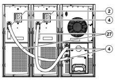
Connect cable **27** to the connectors **4** of the electronic and battery modules.
